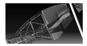
The envelope of a building usually has plenty of space for a structure; for example, with a bridge the size and form of the structure informs the visual design. For Slipstream it was necessary to undergo a three-way iterative design process of controlling the form via the plane's flight path, understanding the volume created, and checking that a structure of adequate strength could fit inside. It took 48 versions to arrive at a form with a structure that could be accommodated.
